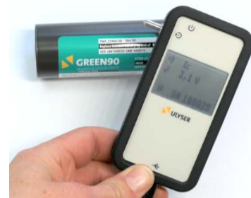
Figure 26: Checking the Acoustic Signal
