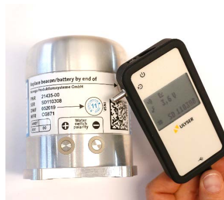
Figure 29: Checking the Acoustic Signal
